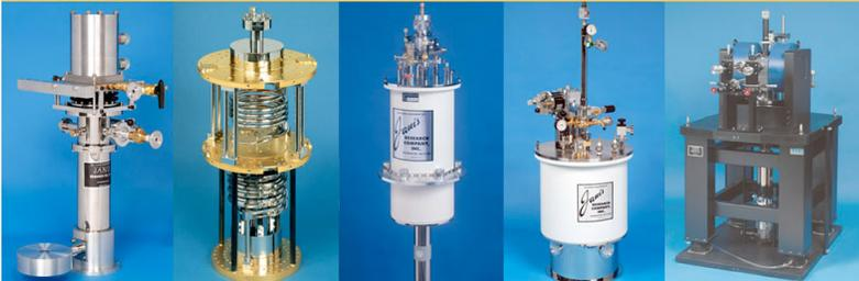
10 mK to 800 K      LHe/LN<sub>2</sub> Cryostats
