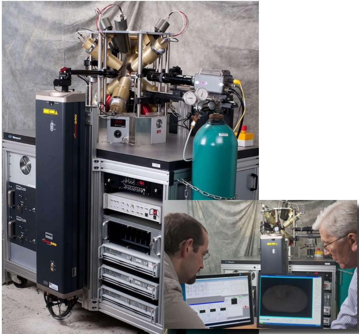
Photograph of the Model 3.1 Aero-Acoustic Levitator system showing table-top levitator, CO 2 laser beam heating, rack-mounted electronics, and Vision Research fast camera.
